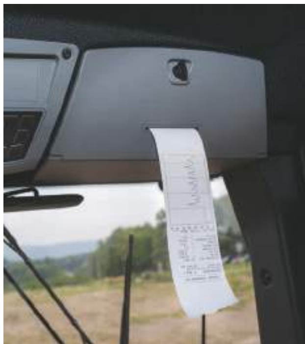
Integrated printer: for documentation of compaction results.
