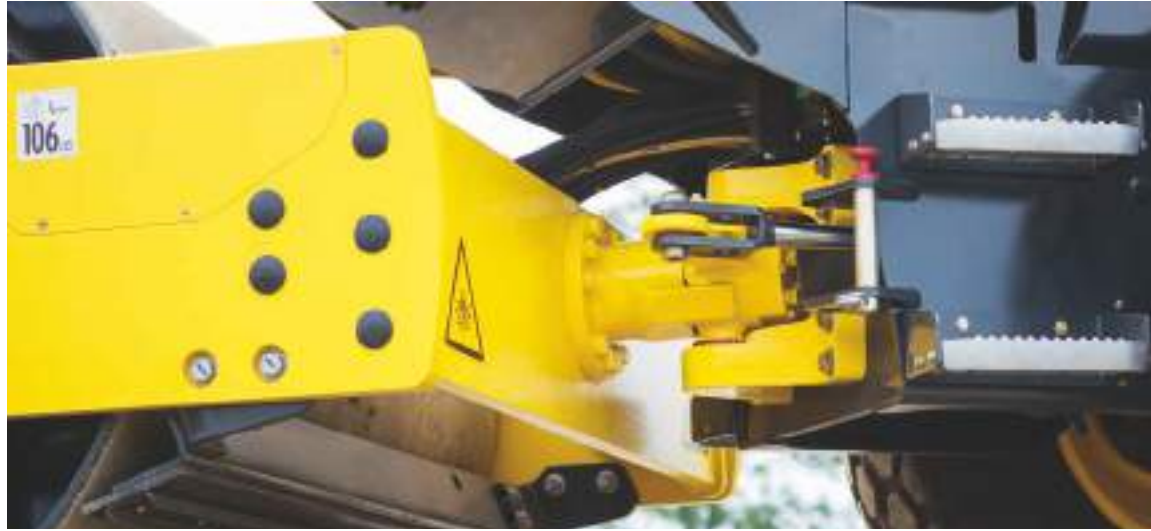
Clean-cut: The articulated joint is maintenance-free; the machine needs no lubrication whatsoever.
