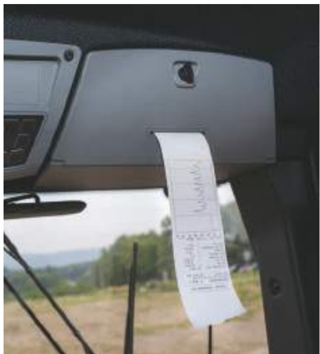
Integrated printer: for documentation of compaction results.
