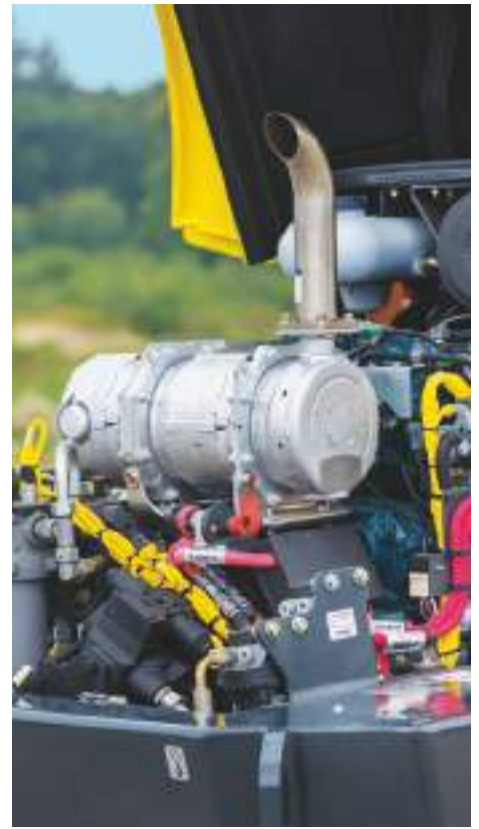
All cables are protected against damage.
