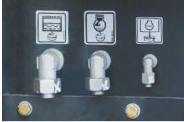
Smart: operating materials can be drained externally.
