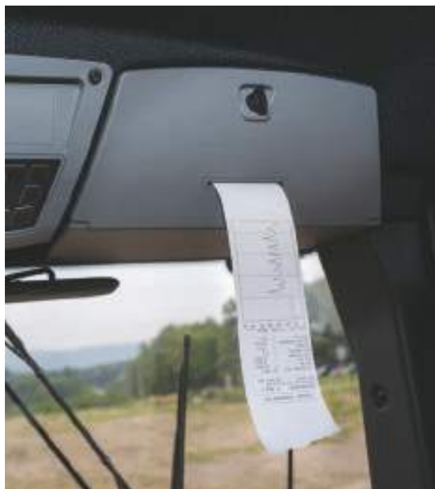
Integrated printer: for documentation of compaction results.
