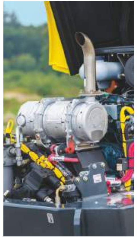
All cables are protected against damage.
